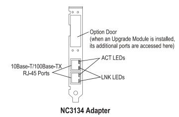
Figure 1-1. NC3134 Server Adapter 10BASE-T/100BASE-TX RJ-45 ports and LED indicators
